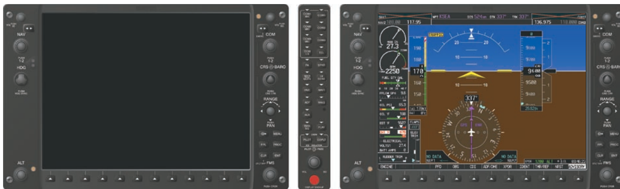
Figure 2.7.2 Reversionary Mode (Failed PFD)
